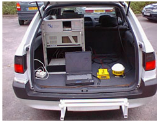
Fig. 5. View of the experimental car with the Ag132 GPS receiver.
