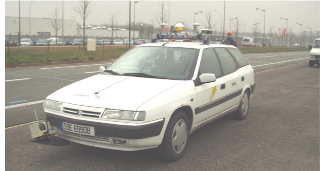
Fig. 4. The experimental car with the Ag132 and Thales GPS receivers
