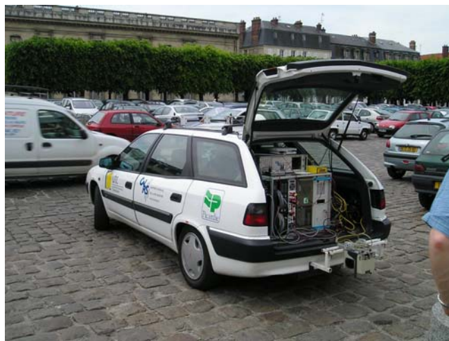
Fig. 10. The Real time acquisition system in STRADA.
