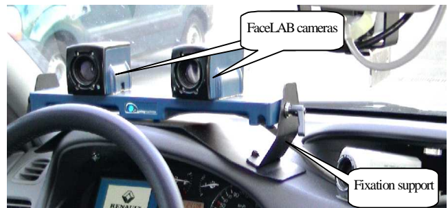
Fig. 4. Overview of the stereo pair cameras of FaceLab in the experimental car.
