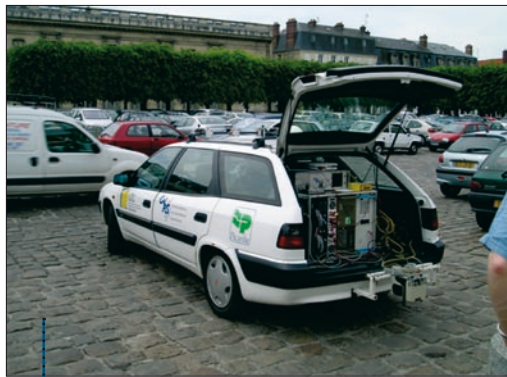
Figure 5 - The Real time acquisition system in STRADA.
