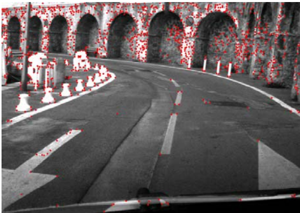
Fig. 2. Example of detected visual features: Harris points
