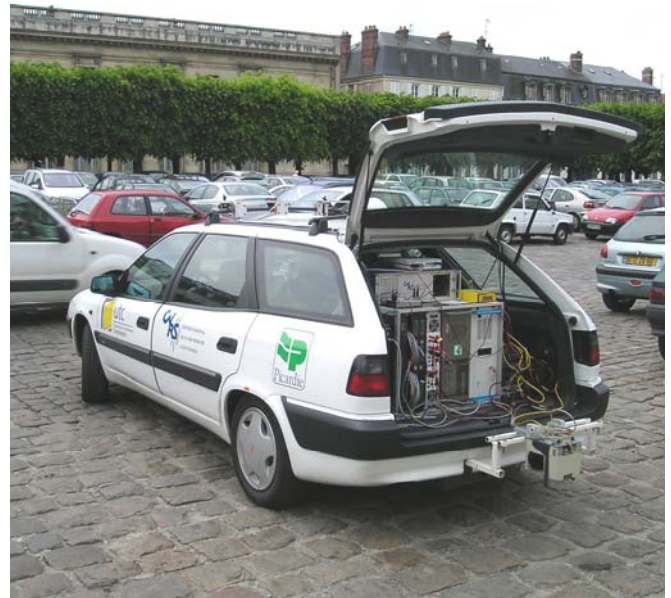
Fig. 1. Experimental car used as a mobile mapmaker.
