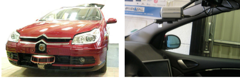
Figure 6. Experimental platform: Lidar (left), Camera (right)
