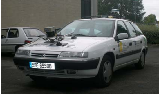
Fig. 1. LMS SICK 291 on the hood of the vehicle
