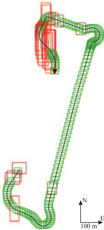
Figure 7: Trajectory. Boxes are bounding boxes of non robust solution sets. Reference trajectory is in black.
