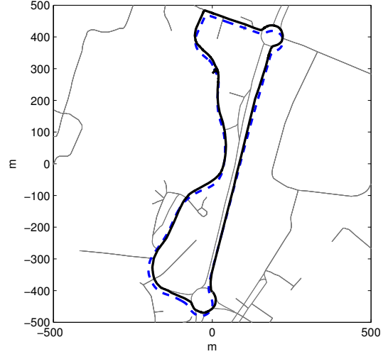
Fig. 2: Trajectory -dashed- vs. map-matched trajectory -plain- in a ENU frame centered on the map.
