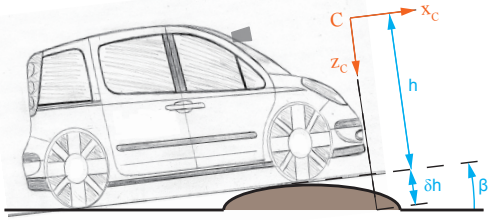
Fig. 2. Parameter variation while climbing a speed bumper
