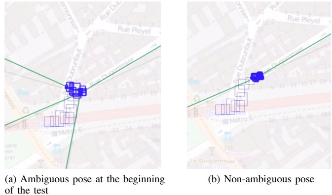
Figure 17. Solution subpaving at two epochs (thick blue boxes). Thin boxes are the position history, green lines point to the used satellites.
