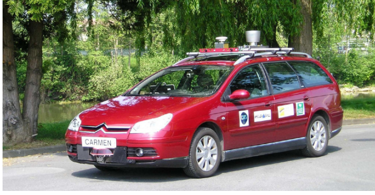
Figure 8: Test vehicle Carmen with the lidar sensor in front.
