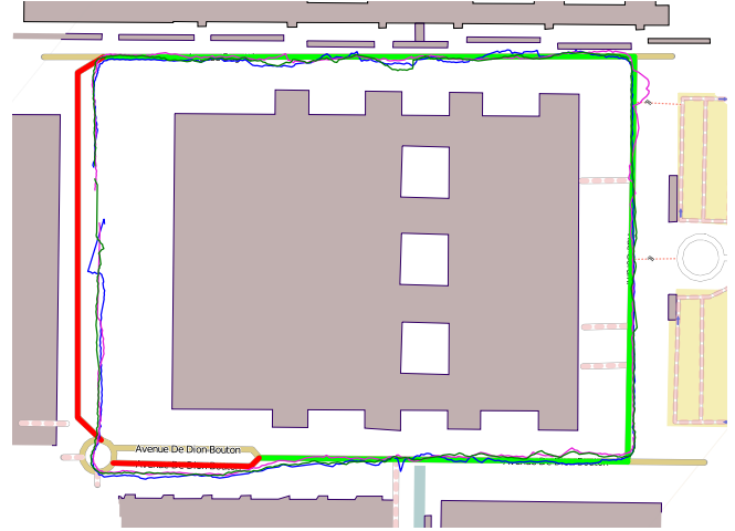
Fig. 6: Results of FDI in a urban environment after three journeys. The red links correspond to map errors that have been fully isolated during the third journey.
