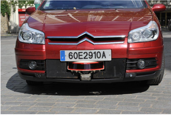
Fig. 4. Vehicle Carmen with Alaska XT lidar embedded in the front bumper.
