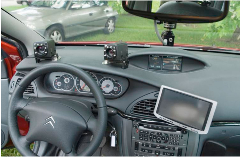
Figure 9.7: Driver interface: active gas pedal, audio, and screen display. The two cameras on the dashboard are used for eye-tracking.
