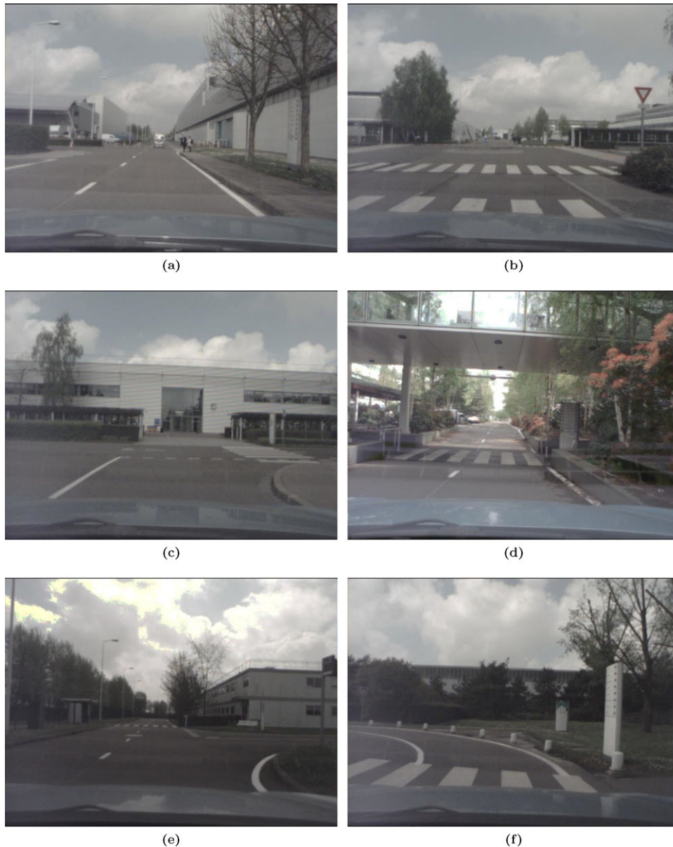
Figure 16. Scenarios recorded by a webcam mounted on the experimental vehicle. The roads in the trials had two lanes with mainly dashed lane markings in the center of the road and solid lane markings on both sides, as in (a). In (b), the vehicle encounters a roundabout with few lane markings. (c) A typical turning scenario: the lane marking detection always fails in such cases. (d) The most challenging situations in our experiments, where multipath effect and camera failure occur at the same time. In (e), the vehicle arrives at a fork where the lane detection fails. In (f), the camera fails to detect the highly curved lane markings. Their positions in the map are tagged in Figure 15.
