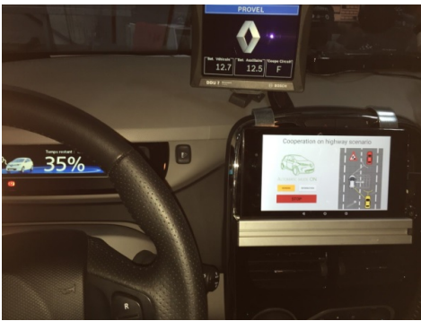
Fig. 6. Human Machine Interface implemented on an Android based tablet.
