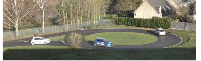
Fig. 10. The experimental “Seville” circuit and the experimental Renault Zoés for the real outdoor tests. In our configuration, the white car (fully autonomous) is the AD vehicle, while the others are the road users (manually driven).
