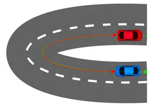
In curved road, compute the inter-distance along the map by using positions exchanged by wireless communication
