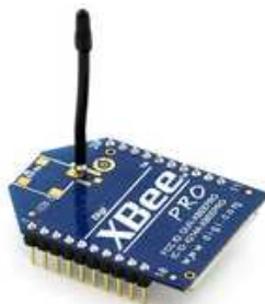
Figure 3.30 – Modem XbeePro . Source : site internet SparkFun [itp].
