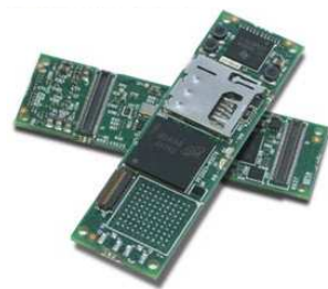
Figure 3.45 – Le Gumstix Overo Water . Source : site Gumstix [ite].
