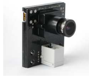
Figure 3.40 – La NXTCam-v2 . Source : site Mindsensors [iti].
