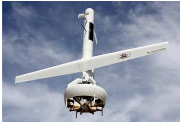
Figure 2.17 – Drone convertible V-Bat de MLB Company . Source : site MLB Company [itj].
