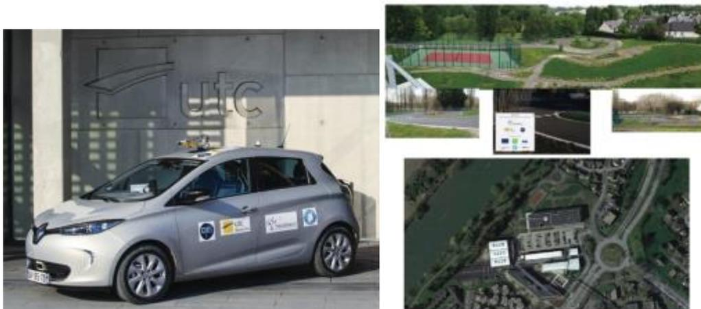
One of the autonomous vehicles based on Renault Zoé cars and the SEVILLE test track
