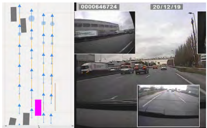
Fig. 3. On the left, tracking results (blue) and measurements (orange for FrontCam, brown for AVM) are displayed in a bird-eye view. On the right, the context cameras.
