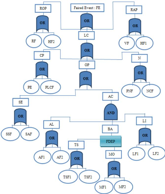
Figure 5. Dynamic Fault Tree of the Moroccan Level Crossing.
