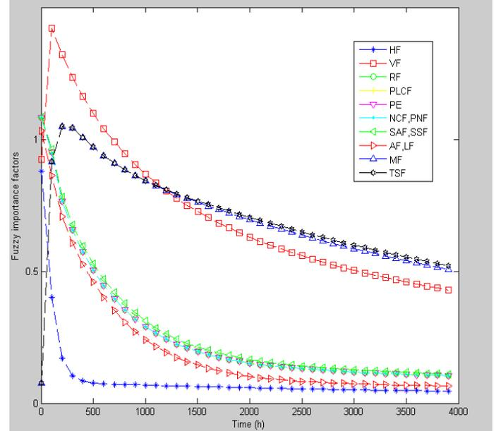
Figure 11. Fuzzy Importance Measures of the level crossing components as a function of time.
