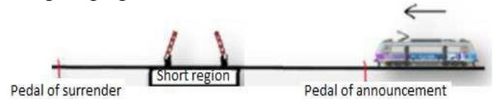
Figure 1. Principle of functioning of the automated level crossing.
