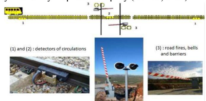
Figure 2. Prototype of the Moroccan Level crossing.
