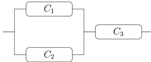
(c) Structure 3: First two component in parallel and the third in series with them
