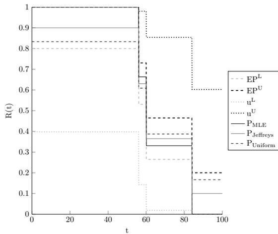
(d) Structure 4: First two component in series and the third in parallel with them
