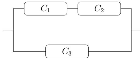
(d) Structure 4: First two component in series and the third in parallel with them
