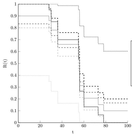
(c) Structure 3: First two component in parallel and the third in series with them
