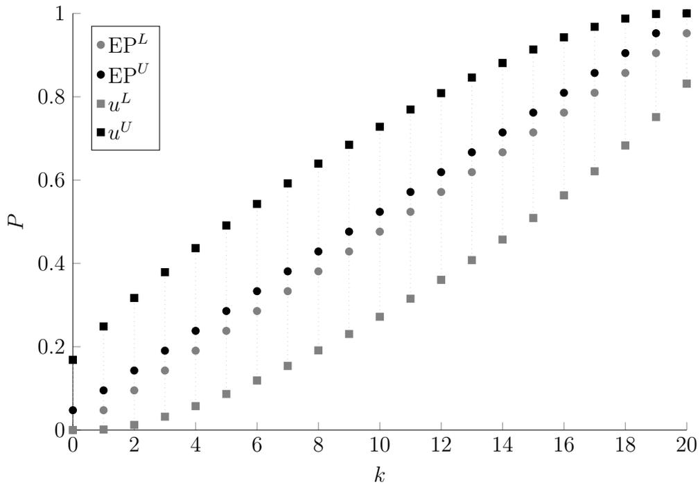
Figure 1: Expected values and confidence intervals of the component failure probability ( $1 - \alpha = 0.95$ ,  $n = 20$ ,  $k = 0 : 20$ )
