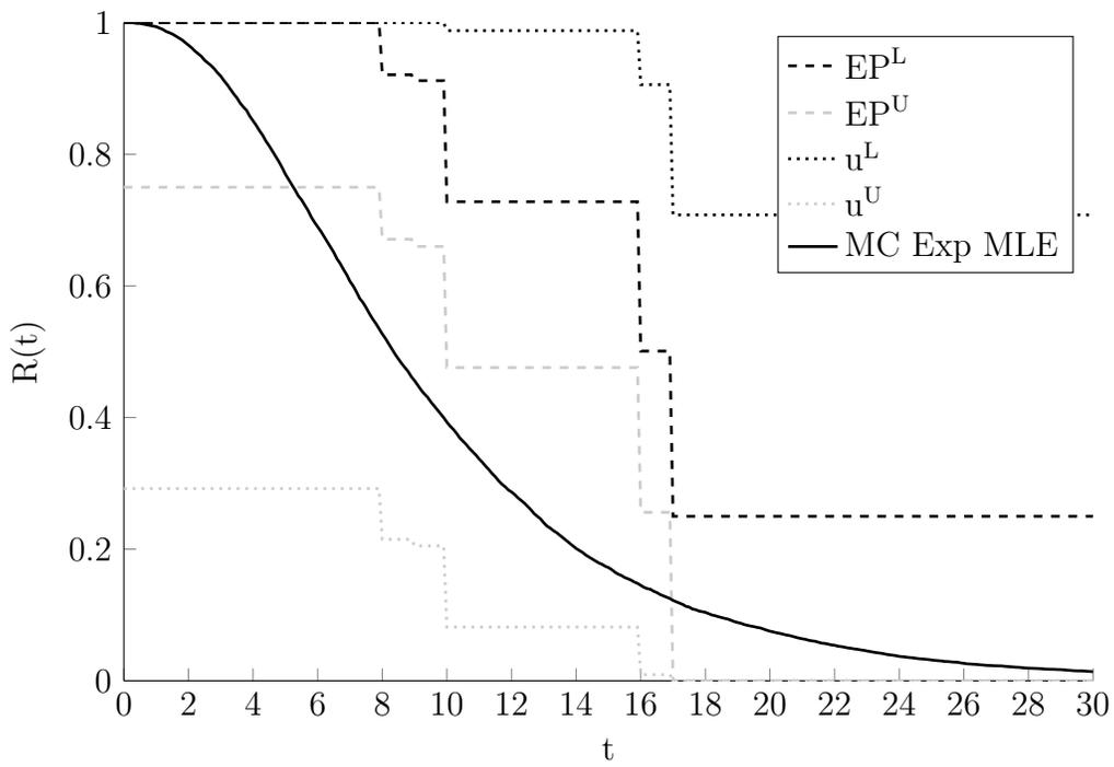
Figure 6: Fault tree BAOBAB2: System reliability  $R_{s,t}$  with  $N = 1000$   $n_s = 3$   $N_{MC} = 10000$
