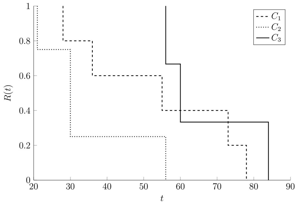
Figure 2: Parallel/serial systems: Empirical reliability for three system components:  $C_1$   $C_2$  and  $C_3$
