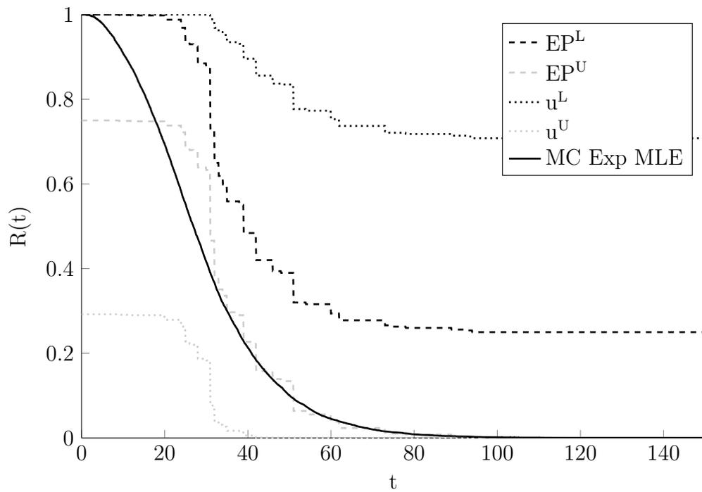
Figure 5: Fault tree BAOBAB1: System reliability  $R_{s,t}$  with  $N = 1000$   $n_s = 3$   $N_{MC} = 10000$
