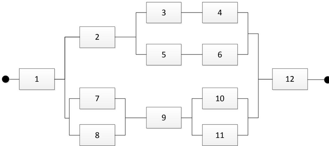
Fig. 12: Reliability block diagram of  $S$ .
