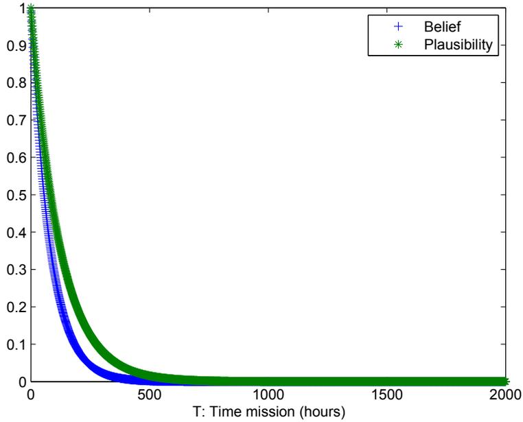
Fig. 9: Belief and Plausibility of the reliability of the airborne control system vs time
