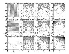
From left to right, the polynomial degree in the kernel increases from 1 to 4; from top to bottom, the first 3 eigenvectors are shown, in order of decreasing eigenvalue size (eigenvalues are normalized to sum to 1).
