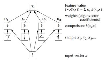
In the first layer, the input vector is compared to the sample via a kernel function, chosen a priori (e.g. polynomial, Gaussian, or sigmoid). The outputs are then linearly combined using weights, which are found by solving an eigenvector problem
