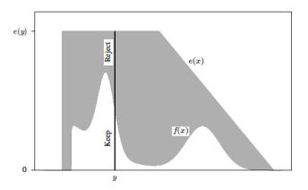
The shaded region above f and below e indicates the waste. The draw Y=y is very likely to be rejected when e(y) is far larger than f(y). Envelopes that exceed f everywhere by at most a slim margin produce fewer wasted (i.e., rejected) draws and correspond to  $\alpha$  values near 1.
