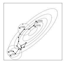
Hypothetical random walk chain for sampling a two-dimensional target distribution (dotted contours) using proposed increments sampled uniformly from a disk centered at the current value.
