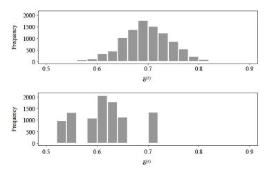
Histograms of  $\delta^{(t)}$  for iterations 201-10,000 of independence chains with proposal densities Beta(1,1) (top) and Beta(2,10) (bottom).
