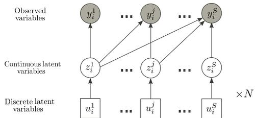
**Fig. 2** Generative model for the diagnosis of track circuits represented by a graphical model
