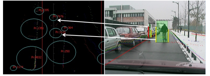
Fig. 1: Object detection system. The figure on the right is an image projection used for the visualization of two objects on the road. The left figure shows the circles encompassing all the detected objects.
