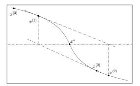
Starting from  $x^{(0)}$ , Newton's method diverges by taking steps that are increasingly distant from the true root,  $x^*$ . In contrast, the bisection method would converge in this case.
