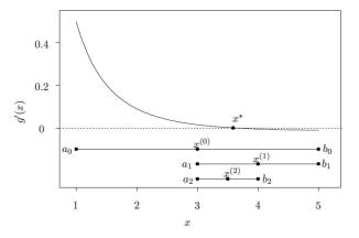
The top portion of this graph shows g'(x) and its root at  $x^*$ . The bottom portion shows the first three intervals obtained using the bisection method with  $(a_0, b_0) = (1, 5)$ . The tth estimate of the root is at the center of the tth interval.
