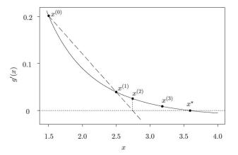
The secant method locally approximates g' using the secant line between  $x^{(0)}$  and  $x^{(1)}$ . The corresponding estimated root,  $x^{(2)}$ , is used with  $x^{(1)}$ to generate the next approximation
